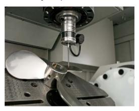
RMP600 high accuracy radio-transmission touch probe
