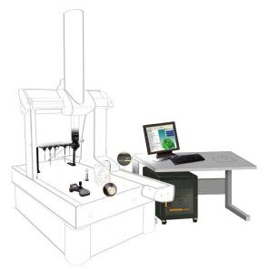
Elements of a CMM retrofit - probe, head, rack, encoders, controller and software
