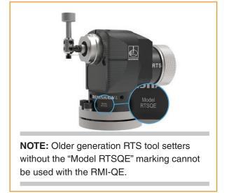
The RTS is a tool setting probe that enables automated broken tool detection and rapid measurement of the tool length and diameter of a wide range of tools, on machining centres of all sizes, or where line-of-sight between probe and receiver is difficult to achieve.
