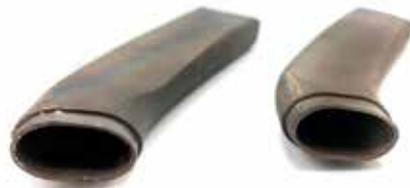
3D printed titanium chainstay bracket component printed on RenAM 500S system
