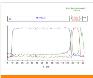
Figure 3. Raman depth profiles from a complex foil-backed polymer laminate.
