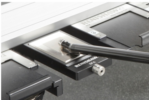
Surface finish cranked stylus on the calibration artefact
